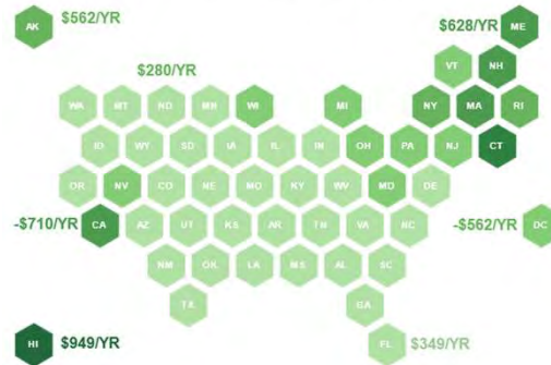
Expected Annual Energy Bill Savings Switching from a 50-gal electric resistance water heater to a 80-gal heat pump water heater
