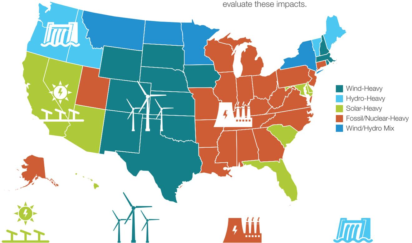
**Solar-Heavy:** PV panels produce more energy during mid-day hours, but grid peak demand often comes later in the day, especially in summer. Consider strategies that enable the building to shift energy away from morning and evening and toward 10am-2pm, such as grid-integrated heat pump water heaters and batteries. Target energy storage duration of 2-8 hours.
