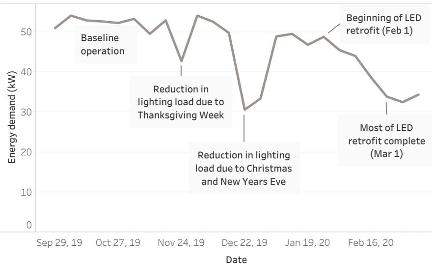
The Welch Hall retrofit demonstrated an impressive whole-building energy reduction of 26% post-retrofit while fully occupied. The lighting energy reduction was 35% and HVAC 29%. These savings are beyond the project expectations. The new LLLC allow the building manager to use the wireless systems to program and fine-tune the lighting and shades based on occupant needs and available daylight. Occupants can always override the settings to make localized adjustments to accommodate their daily needs.
