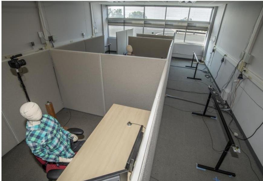
Figure 2. Photograph of INTER system test cell layout. Automated blinds are set to a neutral angle ( $0^\circ$ ) and automated rollershades are deployed at a length of approximately 10 inches. *Source: LBNL*
