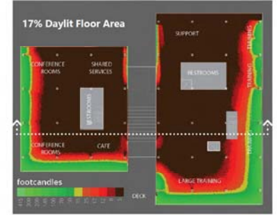
Daylight Illuminance, Uniform Overcast Sky – Mid Floor
