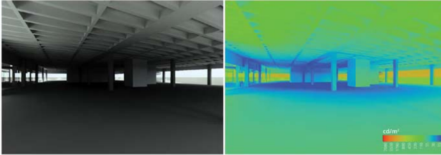
Perspective View and Falsecolor Luminance Map, Equinox at 12pm, Clear Sky with Sun
