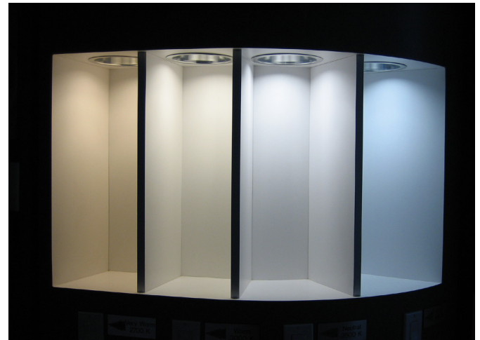
Figure 2: Color temperatures of white light varying 2700K, 3000K, 3500K, and 4100K from left to right. (Image courtesy of the Energy and Technology Center, Sacramento Municipal Utility District.)
