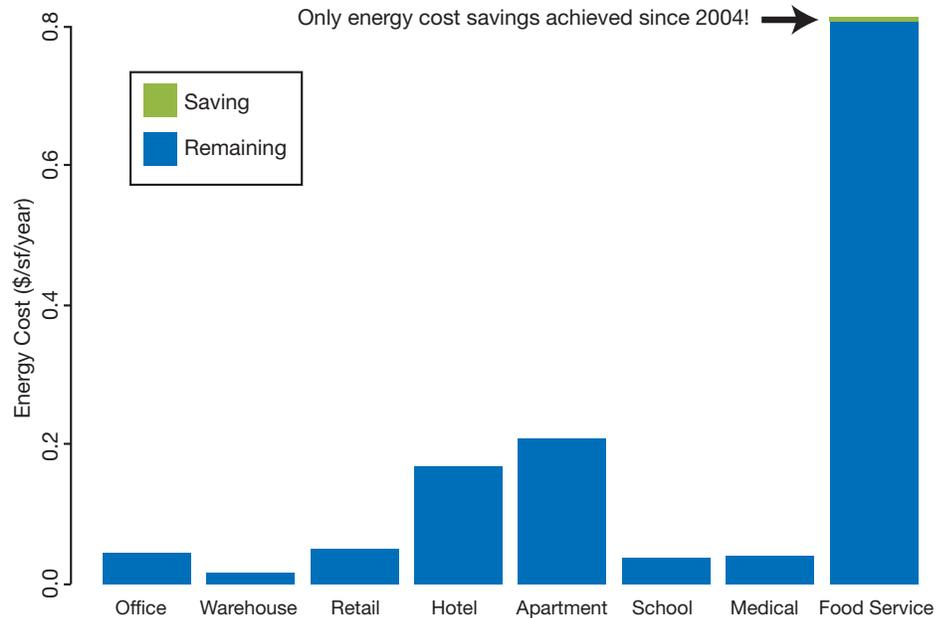
Figure 2: Service hot water: 90.1-2013 vs 90.1-2004; US energy cost<sup>14</sup>
