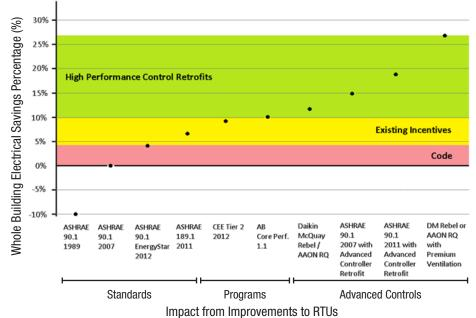
loop at specific conditions, but many performance issues are unrelated to the refrigeration loop. These include power needed to provide ventilation air, the ability to use free cooling, advanced control strategies and fault detection.
